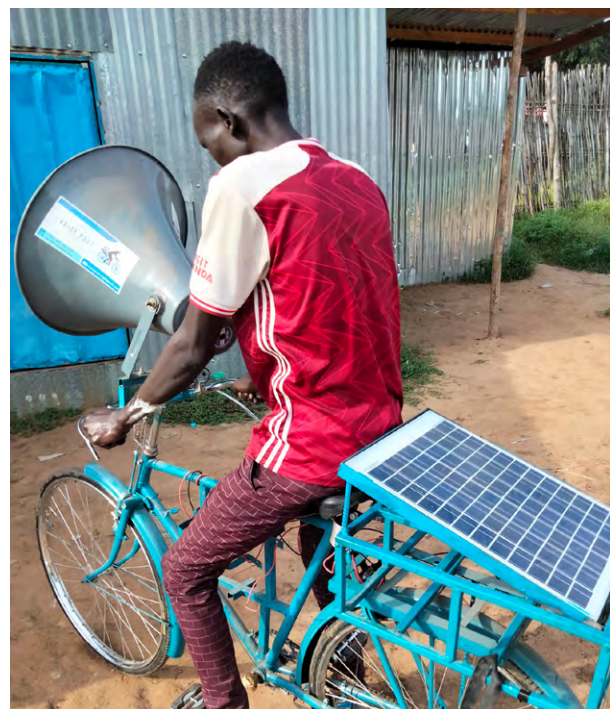
Figure 5. Solar panels installed on a Blue Messenger Bicycle (Credit: Voice Post)
