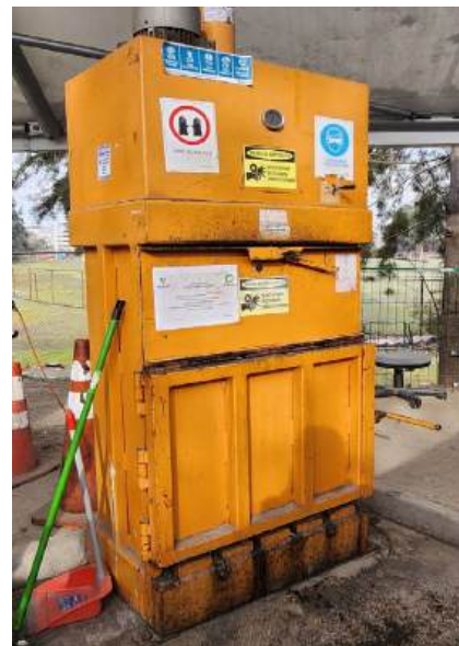
Figure 10. (Above) Two grassroots recyclers sorting PET waste at Serviclaje Cooperative; (left) a drop-off recycling centre for neighbourhood residents to self-sort and dispose of their recyclable waste; (right) a baling press machine used to crush PET waste into bales for ease of recollection (photos by the student research team)
